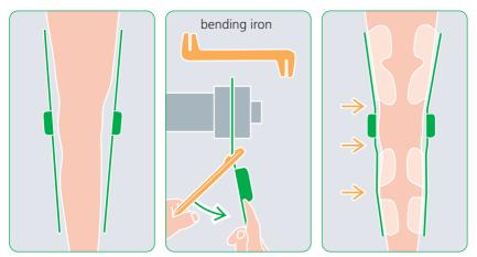
When adjusting the hinge rods to the shape of the extremity by using an orthopaedic bending iron, you must not bend the rods in the area of the hinge housing or the hinge cover as this could lead to damage or break of the hinge.
