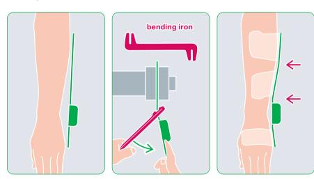
When adjusting the hinge rods to the shape of the extremity by using an orthopaedic bending iron, you must not bend the rods in the area of the hinge housing or the hinge cover as this could lead to damage or break of the hinge.
